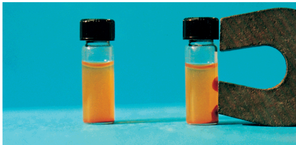
Figure 7. Photograph showing the attraction of the magnetic nanoparticles by a laboratory magnet (right). The right is the result of a control experiment, indicating less settling of the nanoparticles at the bottom of the vial due to gravitational force 6 h after shaking the bottles.
